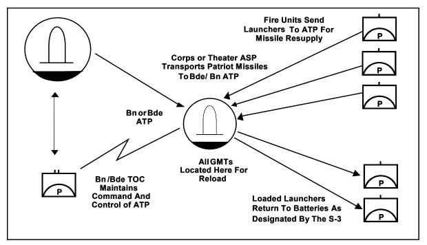
Figure 6-3. Centralized Patriot Missile Resupply
