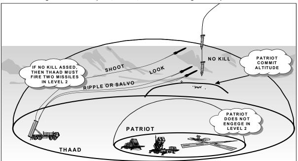
Figure 5-14. Principle 5, Level 2, Patriot Enforcing the Keepout Altitude
