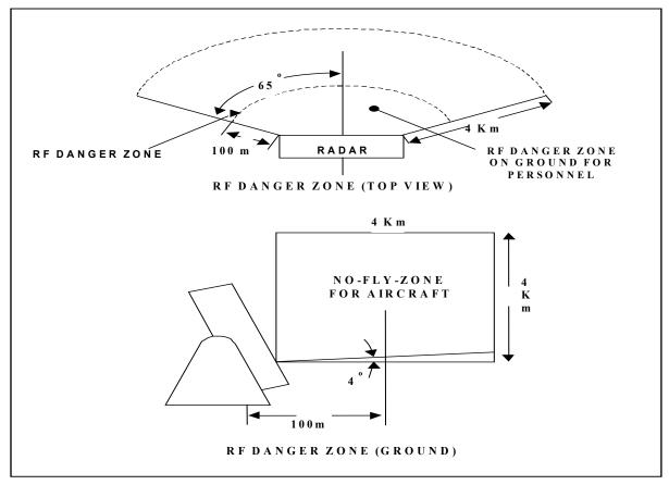
Figure E-2. THAAD Radar RF Hazard Distances
