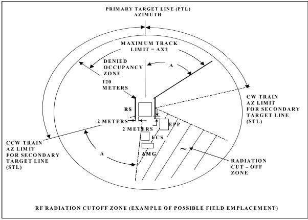
Figure E-1. RF Radiation Hazard
