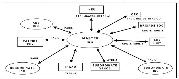
Figure C-18. Data Link Software Capability
