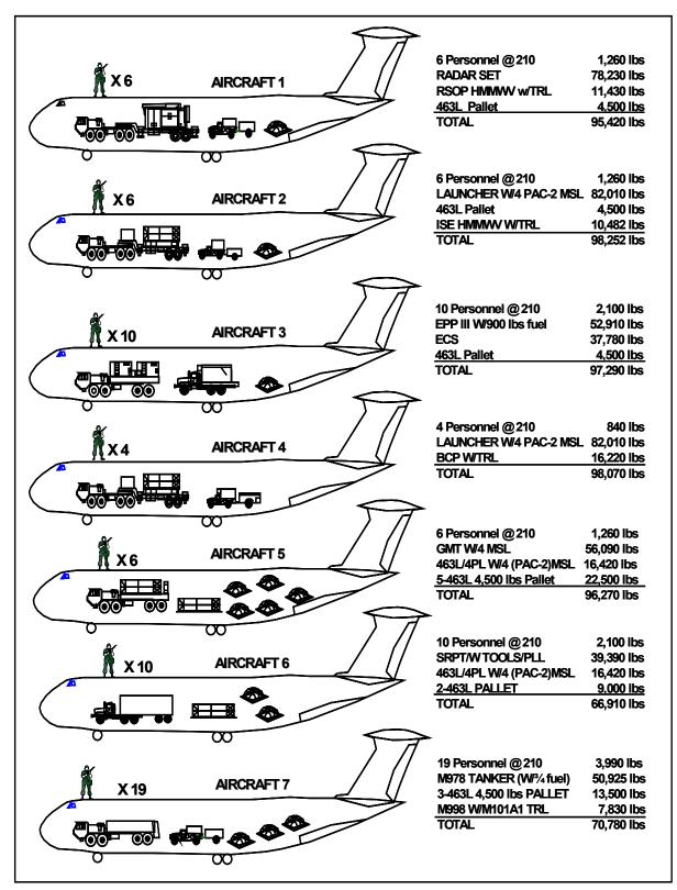
Figure F-3. Allocation of MEP Components on C-17 Aircraft
