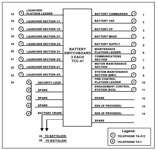
Figure C-9. Battery Switchboard Connections
