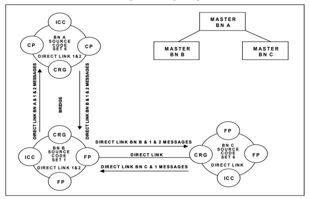
Figure C-17. Direct Linking
